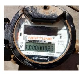
The screen will change, and flow will show as 0.00. Any other numbers on that screen mean that water is flowing at that rate through the meter.
