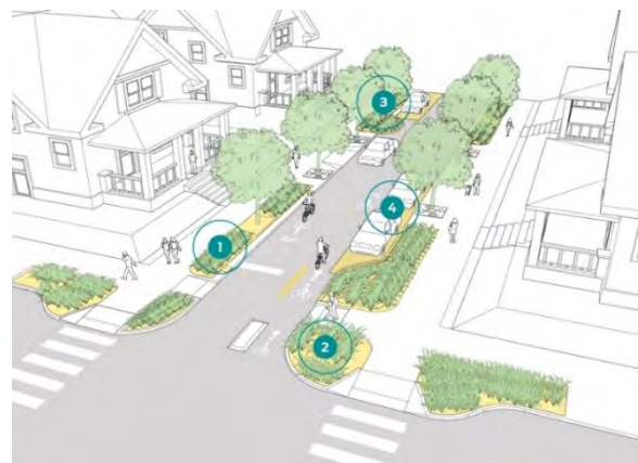
Green street: Vegetated bulb-outs that receive stormwater
